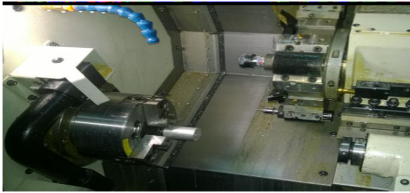
Figure 1: Machining setup used for the HSM of Al 7075 alloy
