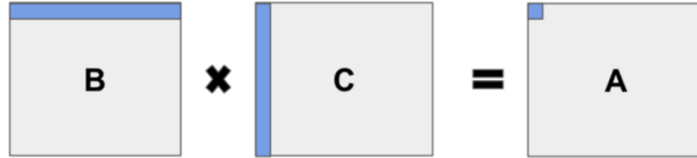
Figure 1: Visualization of standard matrix multiplication process.
