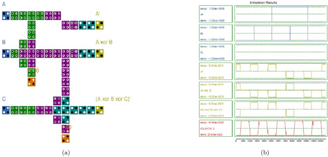
Figure 3: (a) Schematic QCA layout of the projected 3 \times 3 reversible circuit; (b) Simulation results of designed 3 \times 3 reversible circuit
