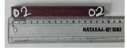
(f) Printed bending test specimen showing scale
